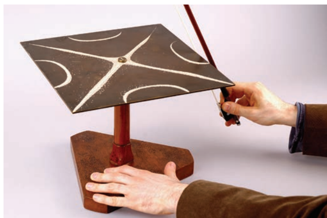
■ Figure C4.21 Demonstrating the oscillations of a metal plate
