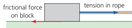
■ Figure A2.22 Frictional force on a block opposing its motion to the right
