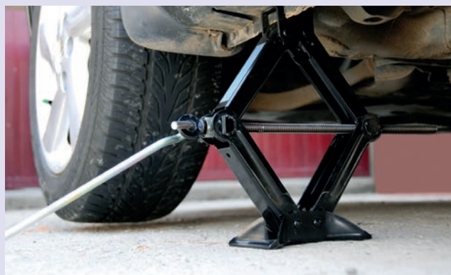
■ Figure A3.25 Changing a car tyre using a simple machine (car jack)
