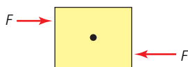
Figure A2.41 The object is in translational equilibrium, but not in rotational equilibrium
