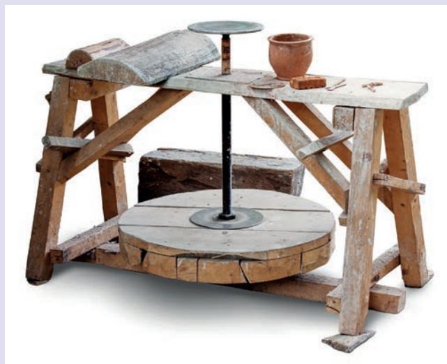
Figure A4.21 A flywheel on a potter’s wheel
