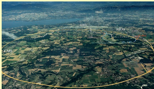
■ Figure D3.12 The Large Hadron Collider at CERN is underground and has a radius of about 4 km
