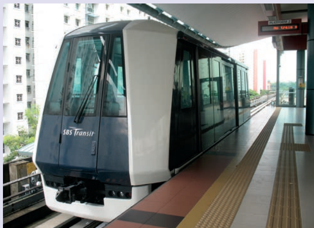
Figure A3.37 The Light Rail Transit trains on the SBS network in Singapore have regenerative braking
