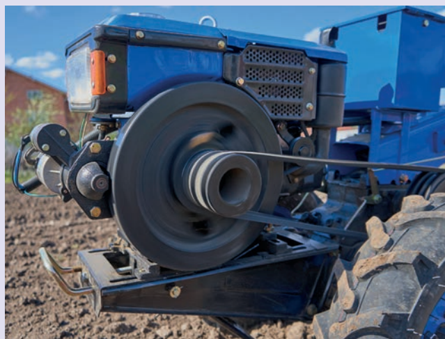
Figure A4.22 Flywheel on a two-wheeled tractor
