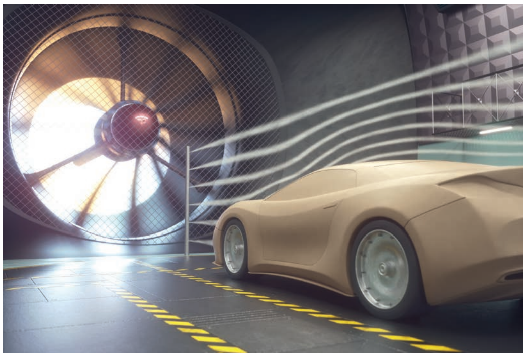
■ Figure A1.44 Air flow over a clay aerodynamic model of a high-performance sports vehicle
