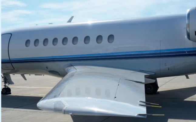
■ Figure D2.20 Static dischargers on the wing of an aircraft
