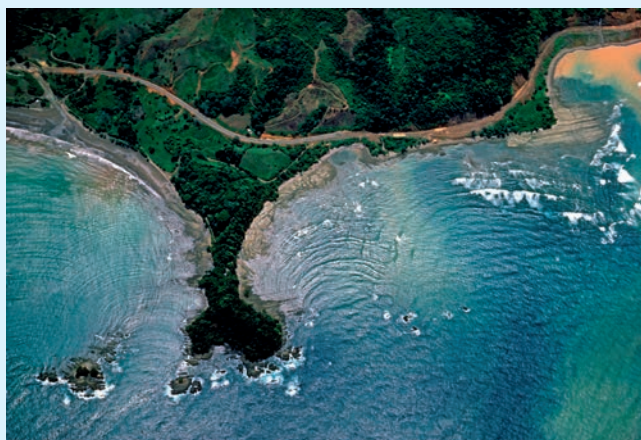
■ Figure C3.5 Ocean waves refracting (and diffracting) as they approach a beach
