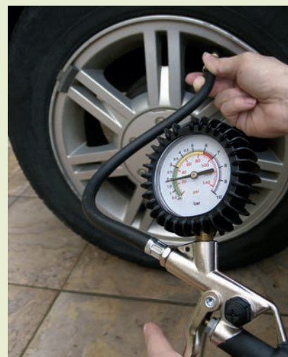
■ Figure B5.11 Measuring the air pressure in a car tyre
