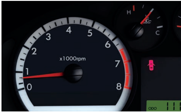
■ Figure A4.10 A car's tachometer displays rpm/1000
